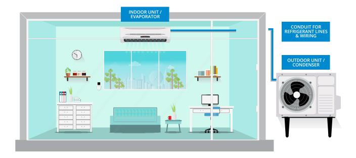
It starts with understanding exactly what ductless mini splits are. Essentially, ductless mini splits are a two-way heating and cooling system, made to transfer hot air outside and, with the help of a compressor and refrigerant, cool the air on its way inside. Each system consists of an outdoor condenser and indoor units placed in multiple locations throughout a building.
